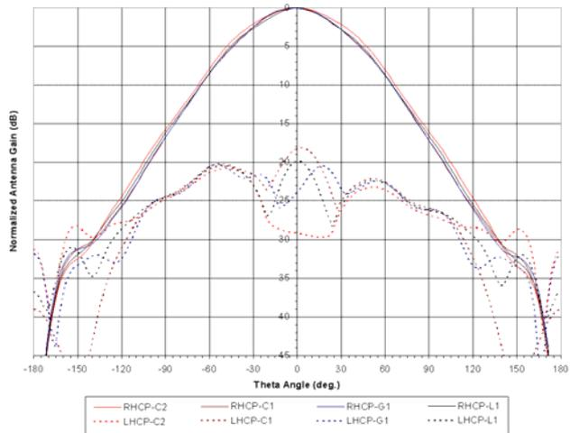
Figure 5: High-band antenna radiation pattern for AT504GG
